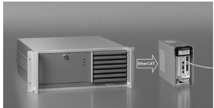
Figure 2: Use of EtherCAT leads to smaller controllers
